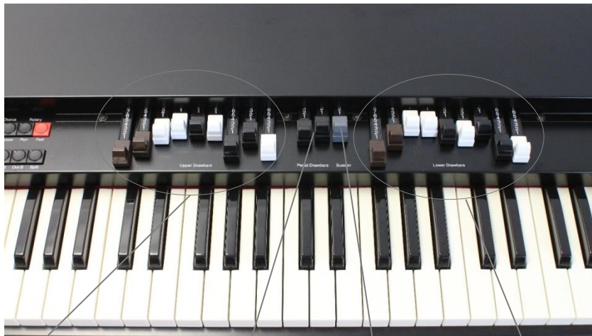
9 Drawbars Upper-Manual 2 Drawbars Bass-Pedal Sustain Bass-Pedal 9 Drawbars Lower-Manual 16" 5 1/3" 8" 4" 2 2/3" 2" 1 3/5" 1 1/3" 1" 16" 8" 16" 5 1/3" 8" 4" 2 2/3" 2" 1 3/5" 1 1/3" 1"
